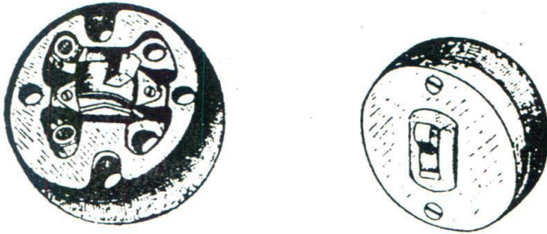
Fig. representing 5 Amp single-way surface switch without cap with moulded box (b) 5 Amp single-way switch with cap (a)
