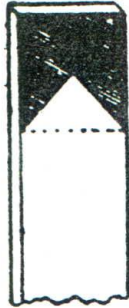
Figure representing top and bottom pieces of capping with the shaded portions marked for removing (c)
