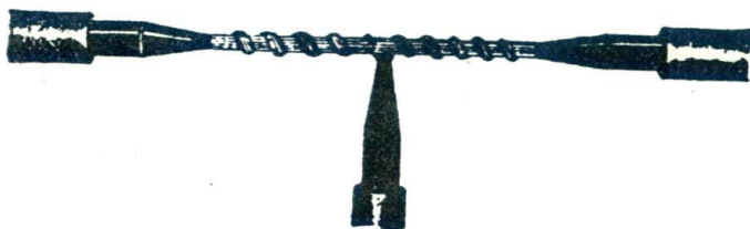
Finished Tap-Joint (c)
