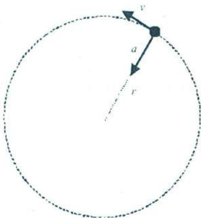
Figure 2.16 An object moving in uniform circular motion due to the centripetal acceleration a .
