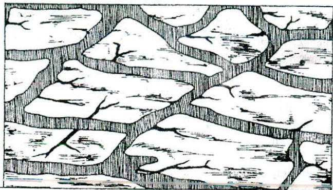
Fig. 22.4. Diagram showing soil cracking due to shrinkage.
