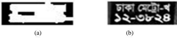
Fig. 8. (a) Result of closing operation, (b) corresponding detected number plate.
