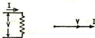
FIG. 9. Resistance branch and vector diagram.
