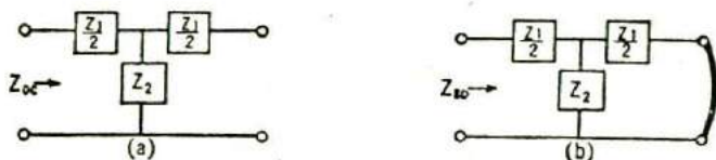
FIG. 5. Z_{o-c} and Z_{s-c} of a symmetrical T-section.
