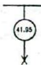
FIG. 14. Resultant percentage of reactance on a 10,000-kva base of Fig. 7 to the point of short circuit.
