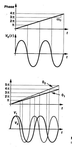
Figure 14.59 Illustration of phase of a signal.
