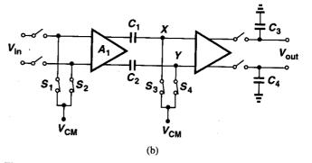
Figure 13.34 (a) Front end of a sampler, (b) circuit of (a) with offset cancellation applied to the first stage.
