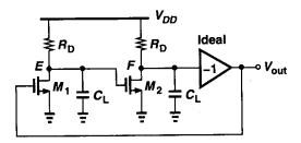
Figure 14.6 Two-pole feedback system with additional signal inversion.
