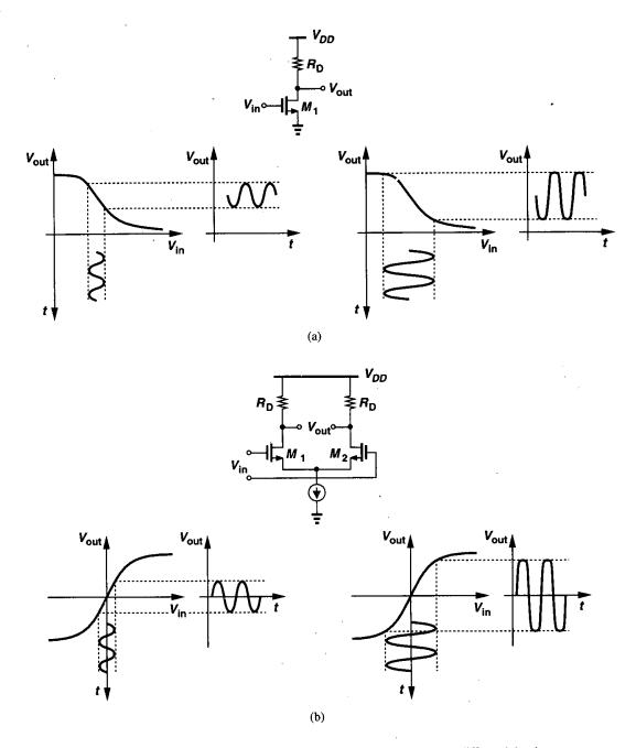
Figure 13.2 Distortion in (a) a common-source stage and (b) a differential pair.
