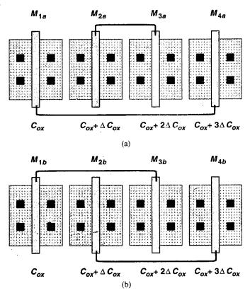
Figure 18.20 One-dimensional cross-coupling.
