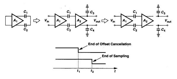
Figure 13.35 Sequence of operations in the sampler.
