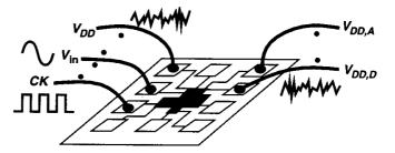
Figure 18.69 Coupling due to mutual inductance between wires.
