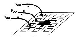
**Figure 18.70** Multiple supply bond wires with mutual coupling.
