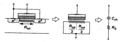
Figure 17.23 Channel resistance of MOS capacitor.
