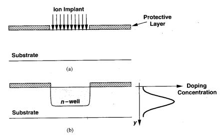
Figure 17.5 (a) Ion implantation, (b) retrograde profile.
