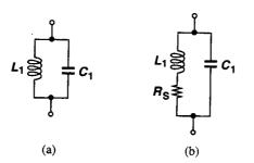
**Figure 14.19** (a) Ideal and (b) realistic LC tanks.
