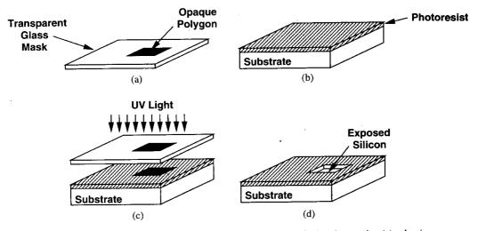
**Figure 17.3** (a) Glass mask used in lithography, (b) coverage of wafer by photoresist, (c) selective exposure of photoresist to UV light, (c) exposed silicon after etching.
