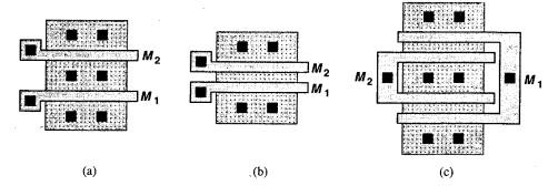
Figure 18.12 Layout of cascode devices having the same width.
