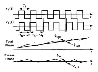
Figure 15.48 Ideal and jittery waveforms.
