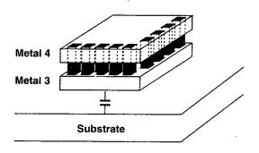
Figure 18.47 Structure of a typical bonding pad.
