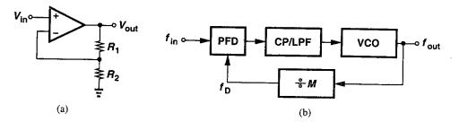
Figure 15.55 (a) Voltage amplification and (b) frequency multiplication.
