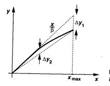
Figure 13.8 Gain error and nonlinearity in a feedback system.
