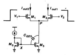
**Figure 18.66** Differential pair operating as a current switch.
