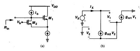
**Figure 14.33** (a) Source follower with positive feedback to create negative input impedance, (b) equivalent circuit of (a) to calculate the input impedance.
