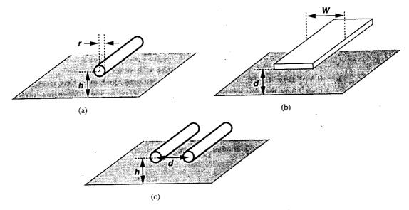
Figure 18.59 Common geometries in packaging.
