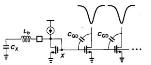
**Figure 18.68** Addition of bypass capacitor externally.
