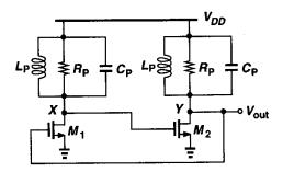
Figure 14.25 Two tuned stages in a feedback loop.
