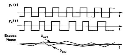
Figure 15.49 Illustration of slow and fast jitter.
