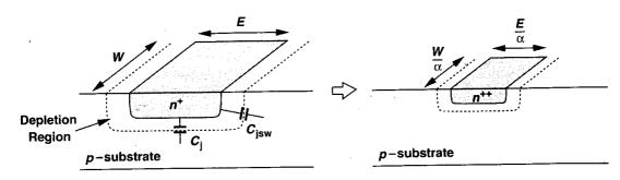
Figure 16.2 Scaling of S/D junction capacitances.
