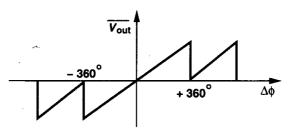
Figure 15.26 Input-output characteristic of the threestate PFD.
