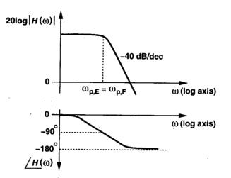
Figure 14.7 Loop gain characteristics of a two-pole system.
