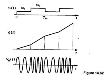
with time at a slope of  $\omega_1$  for half the input period and  $\omega_2$  for the other half. The output waveform of the VCO is similar to that shown in Fig. 14.61. Thus, a VCO can operate as a frequency modulator.
