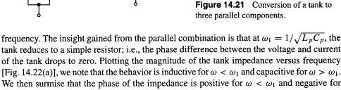
We then surmise that the phase of the impedance is positive for  $\omega < \omega_1$  and negative for  $\omega > \omega_1$  [Fig. 14.22(b)]. These observations prove useful in studying LC oscillators. (Why do we expect the phase shift to approach +90° at very low frequencies and -90° at very high frequencies?)
