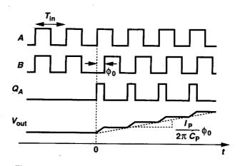
Figure 15.32 Step response of PFD/CP/LPF combination.
