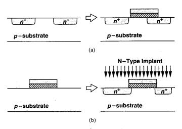
**Figure 17.9** (a) Formation of  $n^+$  regions before deposition of poly, (b) self-aligned structure.
