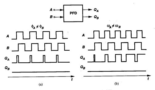
Figure 15.22 Conceptual operation of a PFD.
