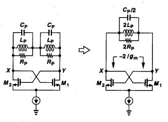
Figure 14.36 Equivalent circuit of Fig. 14.35(b).
