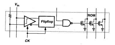
Figure 18.51 A slice of an A/D converter.
