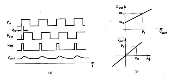
Figure 15.7 (a) Waveforms in a PLL in locked condition, (b) calculation of phase error.
