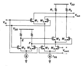
Figure 14.50 Interpolating delay stage with current steering.
