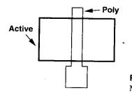
**Figure 17.19** Layout yielding a MOSFET rather than a linear capacitor.
