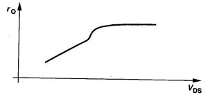
Figure 16.14 Kink in output resistance in Level 3 model.
