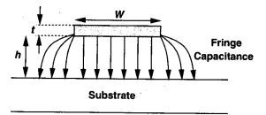
**Figure 17.28** Parallel-plate and fringe capacitance of an interconnect.
