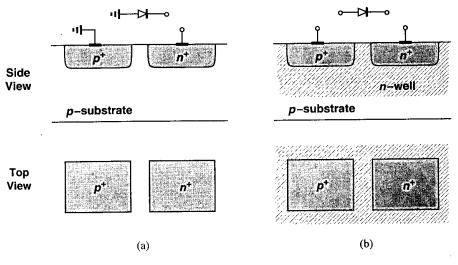
Figure 14.54 Diodes realized in CMOS technology.
