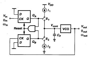
Figure 15.30 Simple charge-pump PLL.
