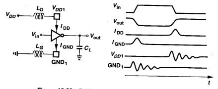
Figure 18.60 CMOS inverter driving a load capacitance.
