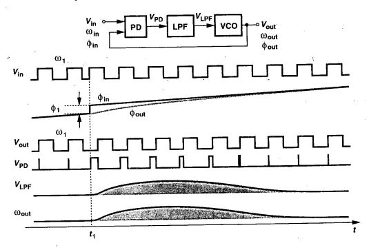
Figure 15.11 Response of a PLL to a phase step.
