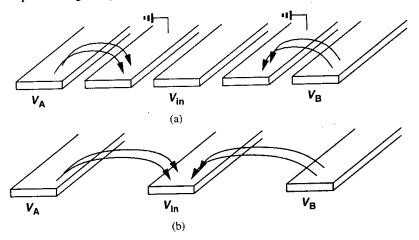
**Figure 18.40** (a) Shielding sensitive signals by additional ground lines, (b) greater spacing between lines to reduce coupling.
