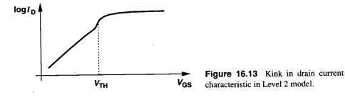
error in representing the output impedance and the transition point between saturation and triode regions. For narrow or long devices, the model is quite inaccurate.
