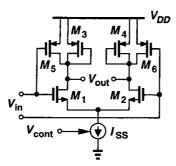
**Figure 14.52** Differential stage with wide tuning range.
