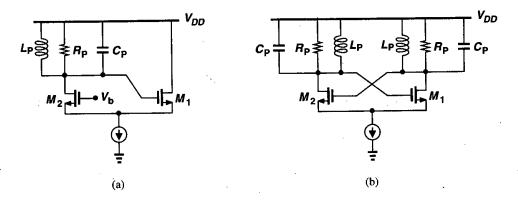
Figure 14.35 (a) Redrawing of the topology shown in Fig. 14.34, (b) differential version of (a).
