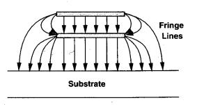
Figure 18.34 Fringe component of capacitance.
