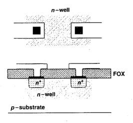
Figure 17.14 Resistor made of *n*-well.
