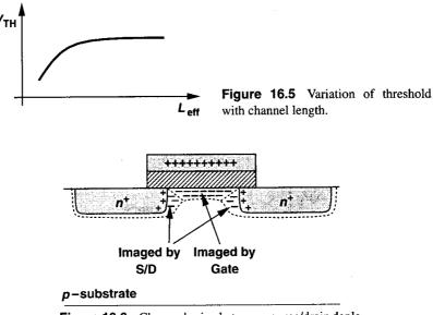
**Figure 16.6** Charge sharing between source/drain depletion regions and the channel depletion region.
