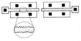
**Figure 13.17** Random mismatches due to microscopic variations in device dimensions.
