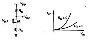
Figure 13.10 Common-source stage with resistive degeneration.
