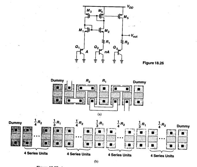
**Figure 18.27** Layout of  $R_1$  and  $R_2$  with (a)  $R_2/R_1 = 5$ , (b)  $R_2/R_1 = 5.34 \approx 16/3$ .
