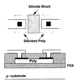
Figure 17.13 Poly resistor using silicide block.
