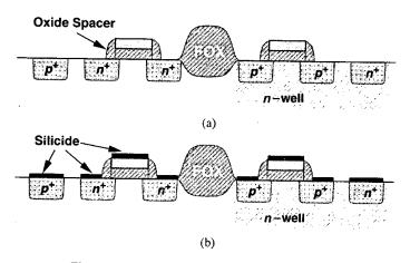
Figure 17.10 (a) Oxide spacers and (b) silicide.
