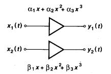
Figure 13.26 Effect of mismatch on second-order distortion.
