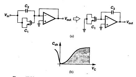
Figure 17.22 Precision multiply-by-two circuit using a MOS capacitor.
