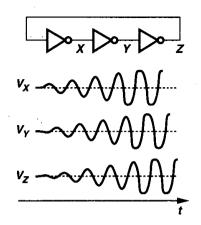
Figure 14.13 Ring oscillator using CMOS inverters.
