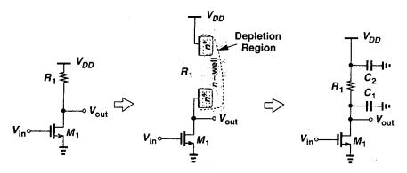
Figure 17.16 Common-source stage using *n*-well resistors.
