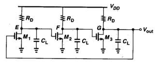
Figure 14.8 Three-stage ring oscillator.
