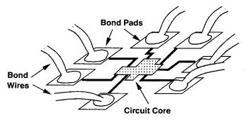
Figure 18.46 Addition of bonding pads to a chip.
