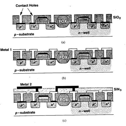
Figure 17.11 Contact and metal fabrication.
