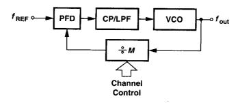
Figure 15.57 Frequency synthesizer.
