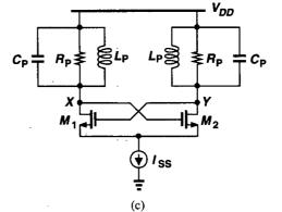
**Figure 14.27** (a) Redrawing of the oscillator shown in Fig. 14.25, (b) another redrawing of the circuit, (c) addition of tail current source to lower supply sensitivity.
