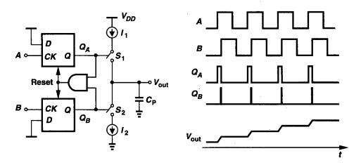
Figure 15.28 PFD with charge pump.
