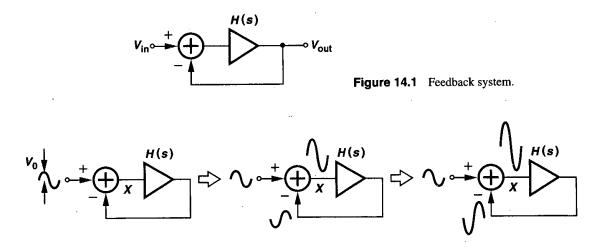
Figure 14.2 Evolution of oscillatory system with time.
