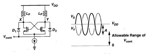
Figure 14.53 LC oscillator using varactor diodes.
