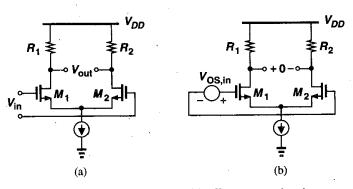
**Figure 13.21** (a) Differential pair with offset measured at the output, (b) circuit of (a) with its offset referred to the input.
