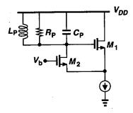
**Figure 14.34** Oscillator using negative input resistance of a source follower with positive feedback.
