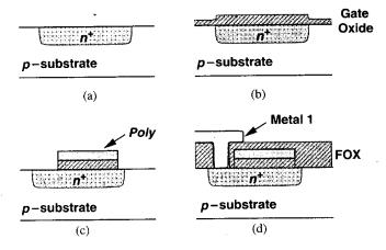
Figure 17.18 Fabrication steps of poly-diffusion capacitor.
