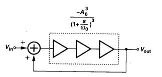
Figure 14.10 Linear model of three-stage ring oscillator.
