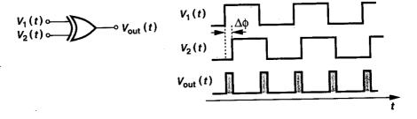
Figure 15.2 Exclusive OR gate as phase detector.
