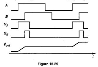
The circuit of Fig. 15.28 has an interesting property. If A, say, leads B by a finite amount,  $Q_A$  produces pulses indefinitely, allowing the charge pump to inject  $I_1$  into  $C_P$  and forcing  $V_{out}$  to rise steadily. In other words, for a finite input error, the output eventually goes to  $+\infty$  or  $-\infty$ , i.e., the "gain" of the circuit is infinity. The consequences of infinite gain are described below.
