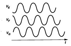
Figure 14.9 Waveforms of a three-stage ring oscillator.
