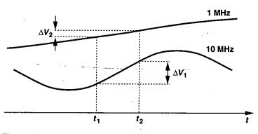
**Figure 13.36** Variation of 1-MHz and 10-MHz noise components in a time interval of 10 ns.
