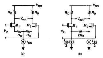
Figure 13.11 Source degeneration applied to a differential pair.
