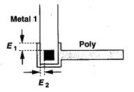
Figure 18.5 Enclosure rule for poly and metal surrounding a contact.
