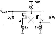
**Figure 14.58** Negative- $G_m$  oscillator using PMOS devices to eliminate n-well capacitance from the tanks.
