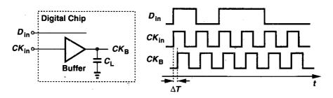
Figure 15.58 Skew between data and buffered clock.
