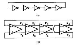
**Figure 14.15** (a) Five-stage single-ended ring oscillator, (b) four-stage differential ring oscillator.
