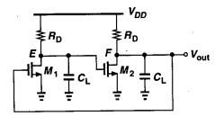
Figure 14.5 Two-pole feedback system.
