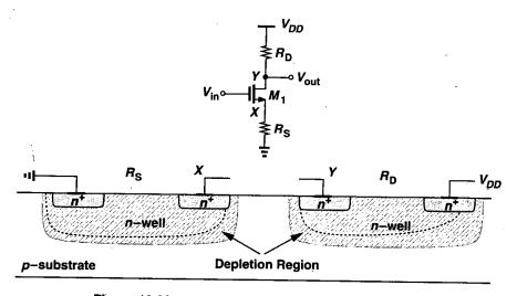
Figure 18.30 Common-source stage using *n*-well resistors.
