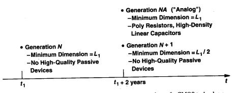
Figure 18.24 Development of digital and analog generations of a CMOS technology.
