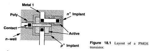
In most modern layout tools, the implants, and even the n-wells are automatically generated from the remainder of transistor geometries, reducing the number of layers that the layout designer sees on the computer screen and simplifying the task.
