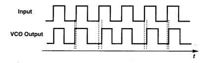
**Figure 15.42** Jitter resulting from the dead zone.
