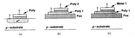
Figure 17.17 Linear capacitor structures, (a) poly-diffusion, (b) poly-poly, (c) metal-poly.
