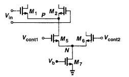
**Figure 14.46** Headroom calculation for a current-steering topology.
