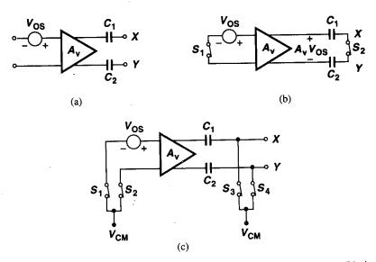
**Figure 13.27** (a) Simple amplifier with capacitive coupling at the output, (b) circuit of (a) with its inputs and outputs shorted, (c) proper setting of the common-mode level during offset cancellation.
