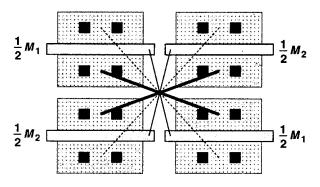
Figure 18.19 Common-centroid layout.
