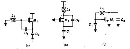
Figure 14.38 Oscillator topologies derived from the circuit of Fig. 14.37(c).
