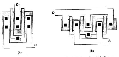
Figure 18.9 (a) Simple folding of a MOSFET, (b) use of multiple fingers.
