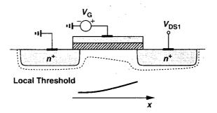
Figure 16.12 Variation of threshold along the channel.
