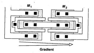
Figure 18.18 Effect of gradient in a differential pair.
