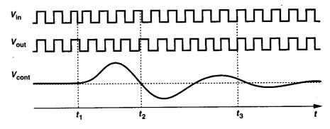
Figure 15.13 Example of phase step response.
