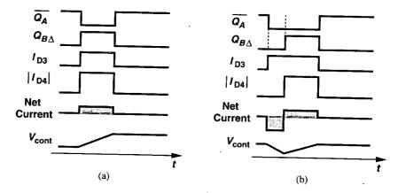
Figure 15.45 Effect of UP and DOWN current mismatch.
