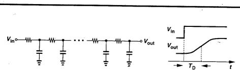
Figure 18.43 Delay and dispersion of a signal in a long line.
