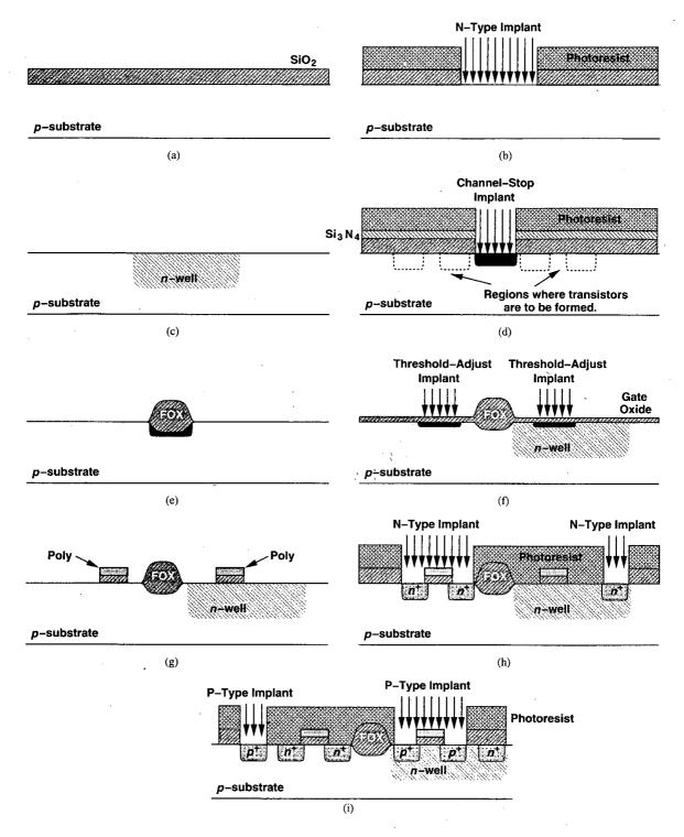
Figure 17.8 Fabrication sequence of MOS devices.
