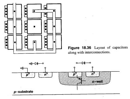
Figure 18.37 Diodes in CMOS technology.
