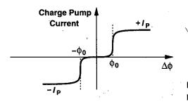
Figure 15.41 Dead zone in the charge pump current.
