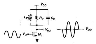
Figure 14.24 Output signal levels in a tuned stage.
