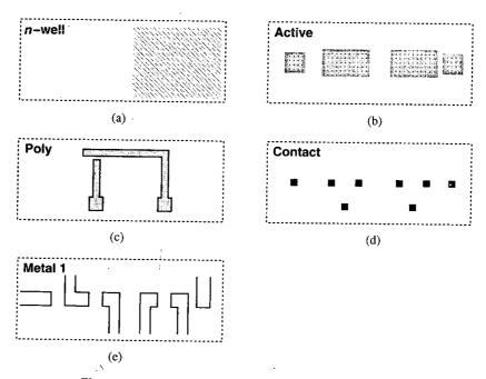
Figure 17.2 Layers comprising the structures of Fig. 17.1.
