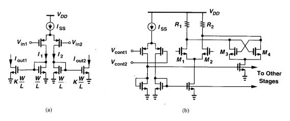
Figure 14.47 (a) Current folding topology, (b) application of current folding to current steering.
