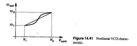
by (14.61), implying that, for a given tuning range, nonlinearity inevitably leads to higher sensitivity for some region of the characteristic.
