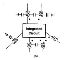
**Figure 18.58** (a) Dual-in-line package, (b) electrical model of the package.
