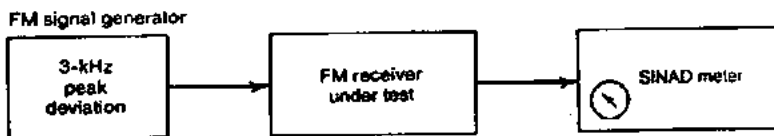
Figure 7.3 Measuring receiver sensitivity.
