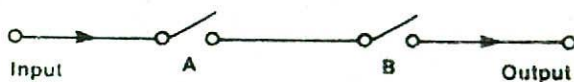
Figure 6.1. Two or more switches connected in series behave as an AND gate.
