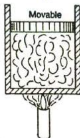
Fig. 2.2. Heat being supplied at constant pressure.
