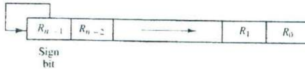
Figure 4-11 Arithmetic shift right.
