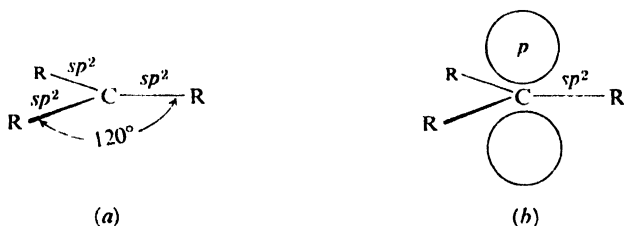
Figure 5.8. A carbonium ion. (a) Only \sigma bonds shown. (b) Empty p orbital above and below plane of \sigma bonds.
