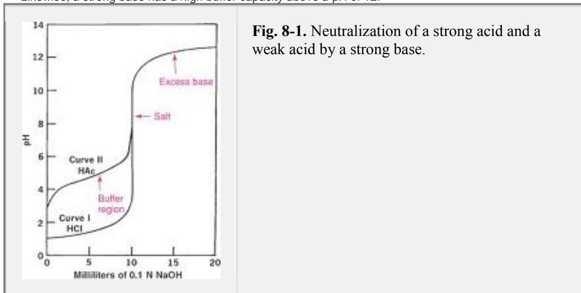
**Fig. 8-1.** Neutralization of a strong acid and a weak acid by a strong base.
