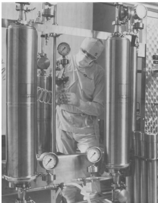
Figure 40-20. An example of a process filtration system in a pharmaceutical plant (courtesy, Millipore).
