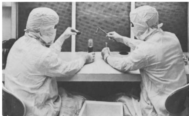
Figure 40-28. Sterility testing of plastic disposable syringes in a horizontal laminar-airflow bench (courtesy, Becton Dickinson & Co).
