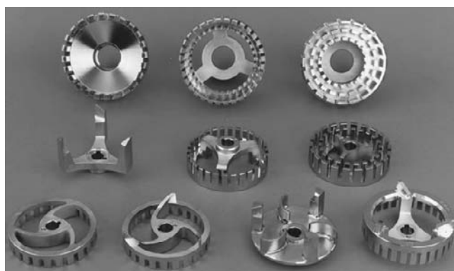
Figure 39-4. Types of rotors used in colloid mills. These may be smooth (for most emulsions), serrated (for ointments and very viscous products), or of vitrified stone (for the paints and pigment dispersions) (courtesy, Tri-Homo).
