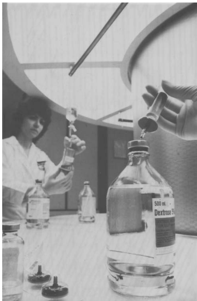
Figure 40-22. Intravenous additive filtration and sterility testing. Both procedures employ membrane filtration (courtesy, Millipore).
