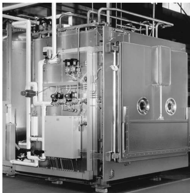
Figure 41-30. Example of a production freeze-dryer (courtesy, Edwards). See Color Plate 16.
