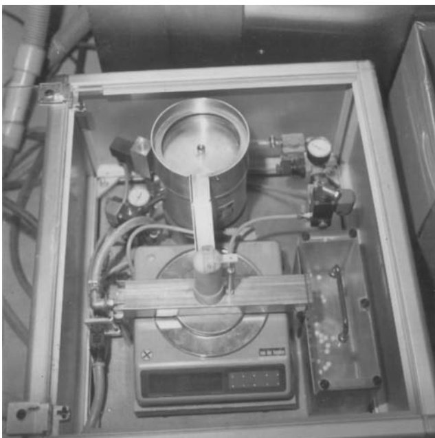
Figure 45-28. Direct weighing of tablets produced gives actual weight feedback for the controller of the Courtoy R-100 (seen in the bottom left of Fig 45-27).
