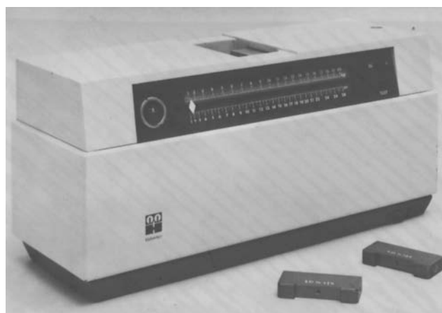
Figure 45-36. The Schleuniger or Heberlein tablet hardness tester shown with calibration blocks (courtesy, Vector).
