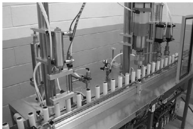
Figure 50-11. Aerosol filling and packaging Terco line for Topical Aerosols (courtesy, Sciarra Laboratories, Inc.)
