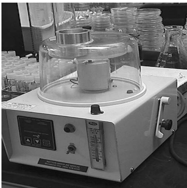
Figure 41-14. Example of slit-to-air sampler (courtesy, Baxter).
