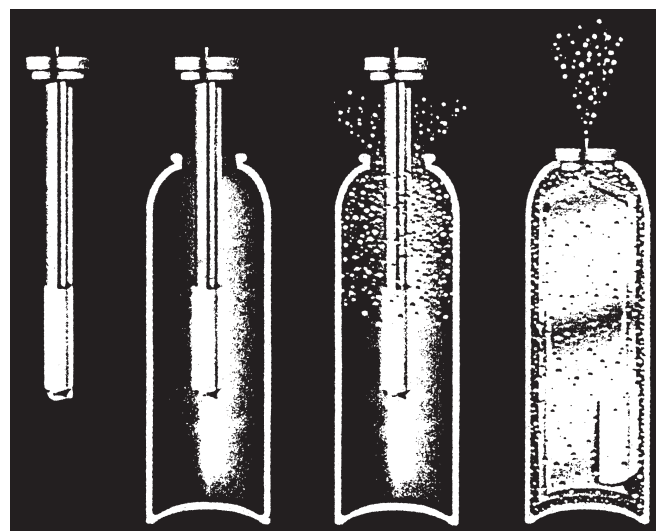
Figure 50-5. Bag-in Can System—ABS (courtesy, CCL Container, Aerosol Division).
