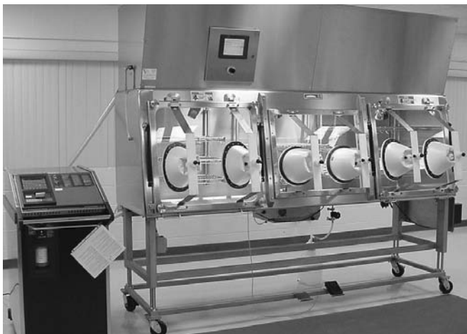
Figure 41-32. Example of an isolator used for sterility testing (courtesy, Baxter). See Color Plate 18.
