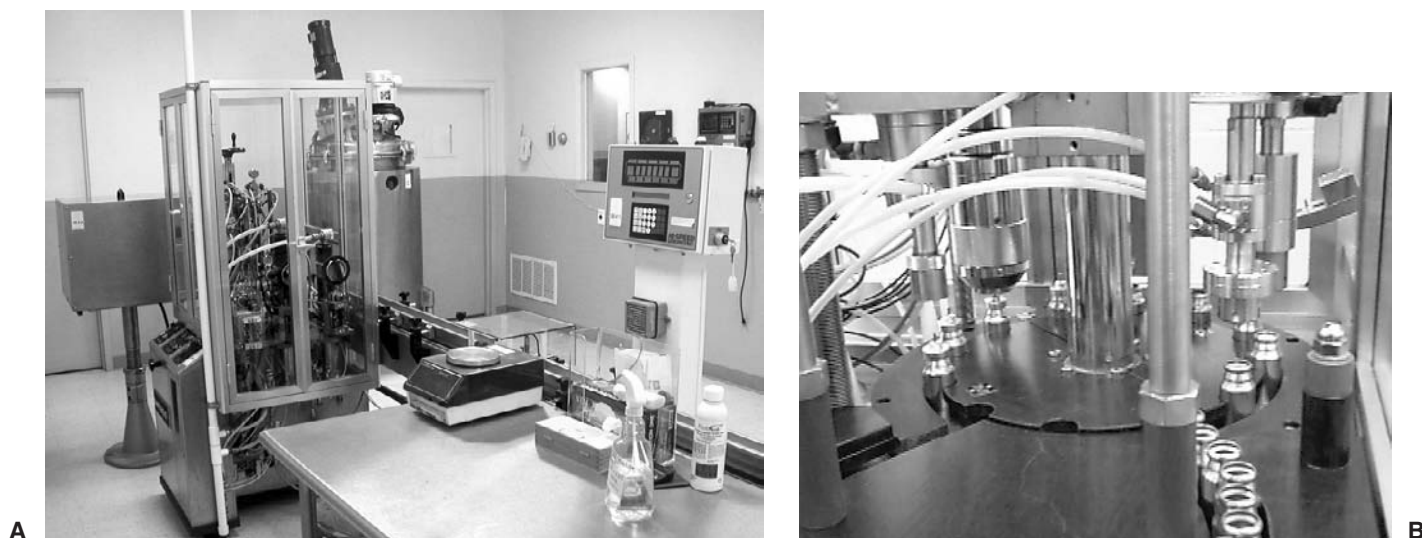
Figure 50-10. (A) Commercial Aerosol filling and packaging Pamasol line for MDIs (courtesy, Sciarra Laboratories, Inc.) (B) Detail of crimping and pressure filling head.
