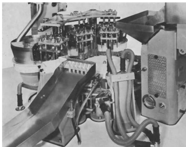
Figure 45-47. Zanasi automatic filling machine, Model AZ-60. The set of filling heads shown at the left collects the powder from the hopper, compresses it into a soft slug, and inserts it into the bottom half of the capsule (courtesy, United Machinery).
