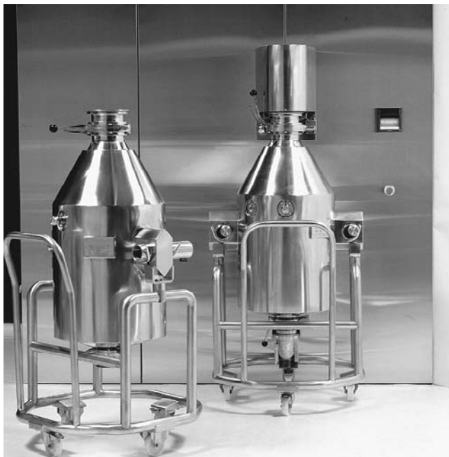
Figure 41-18. Rubber closure processors (courtesy, Getinge USA). See Color Plate 9.
