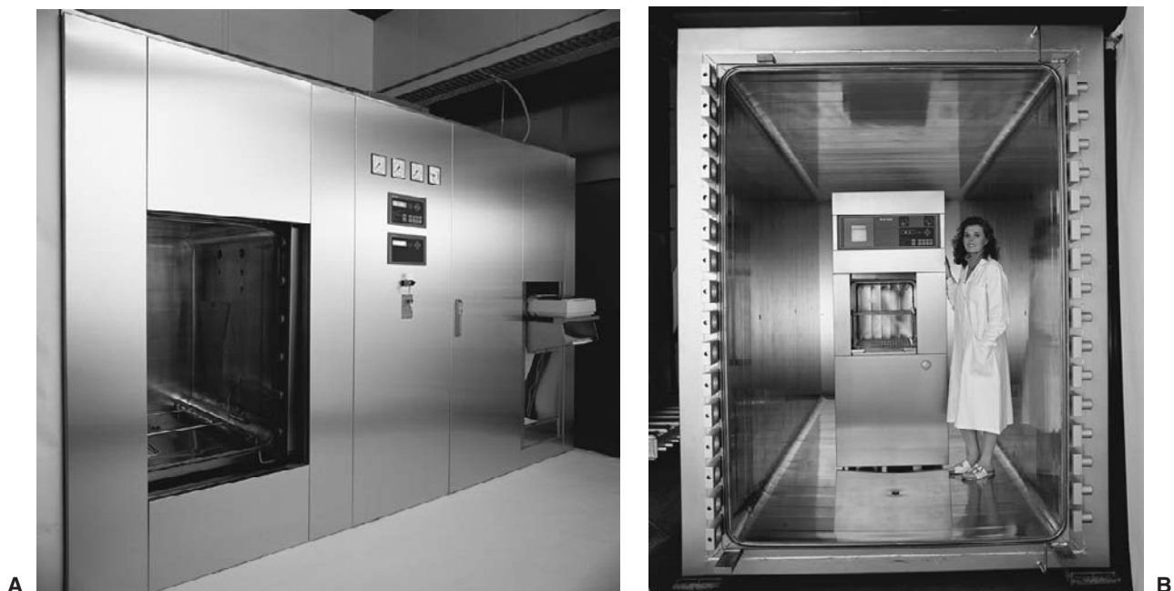
Figure 41-27. Steam sterilizers (small and large) (courtesy, Getinge). See Color Plate 13.
