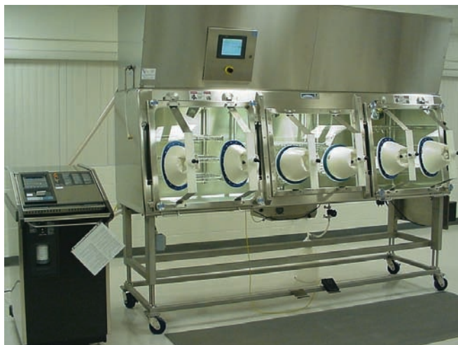
Color Plate 18. Figure 41-32. Example of an isolator used for sterility testing (courtesy, Baxter).
