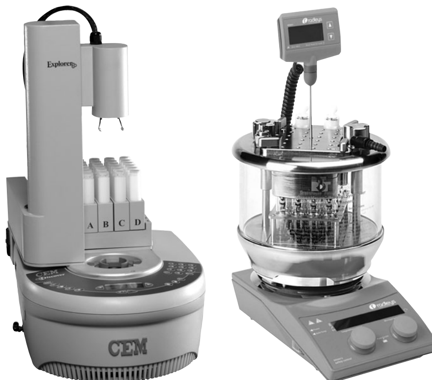
FIGURE 16.15 Laboratory stations for microwave-assisted organic reactions (CEM Explorer-24) and parallel synthesis (Radley's Greenhouse).
