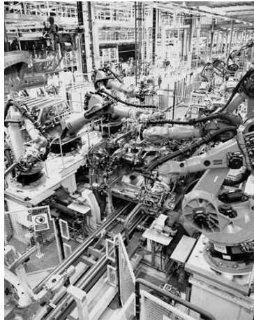
Figure 22.1 Robot arms assembling a car. (Photo courtesy of KUKA Schweissanlagen GmbH in Augsburg, Germany)
